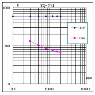
Fig.3 sensitivity characteristics of the MQ-2 14
